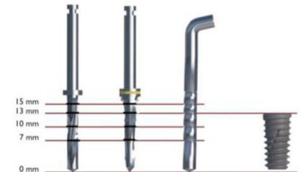
Note: The marks on Twist Drills and Stopper Taper Drills indicate actual millimeter length and correspond to the implant collar. Final vertical positioning depends on several parameters, including esthetics, tissue thickness and available vertical space.
